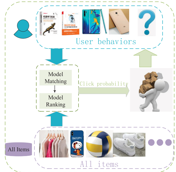
FIGURE 1. Description of running process of the advertising system. In the advertising system, related candidate ad lists are generated for users via methods such as collaborative filtering, and the top recommendations are selected according to the click-through rate to the user.
