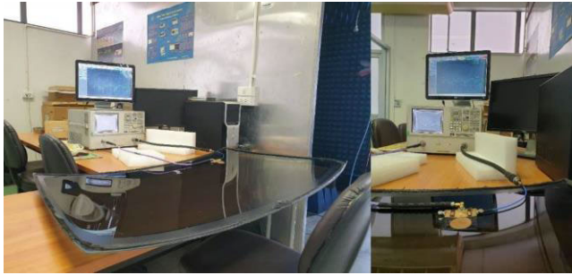
FIGURE 25. Performing measurements on the antenna’s characteristics as installed on the windshield.
