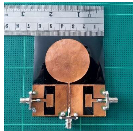
FIGURE 14. The prototype structure of the proposed UWB MIMO antenna.
