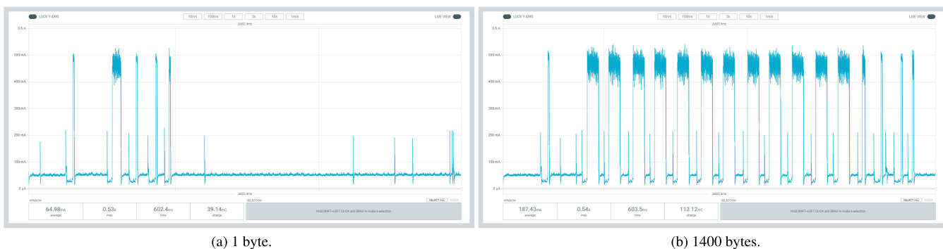
FIGURE 11. NB-IoT UDP transmission close up.
