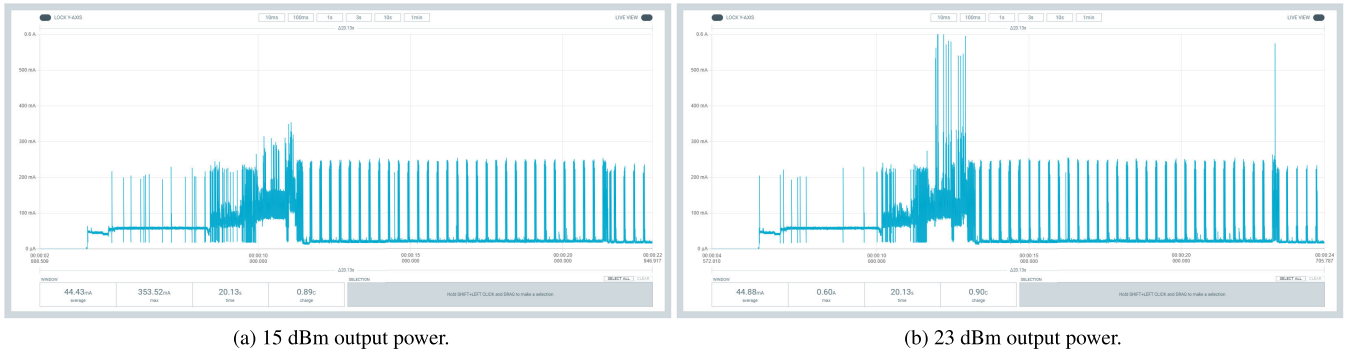
FIGURE 5. eMTC boot up with C-DRX.
