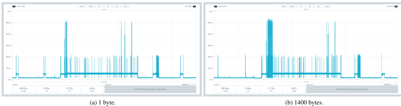
FIGURE 10. NB-IoT sending a UDP payload.
