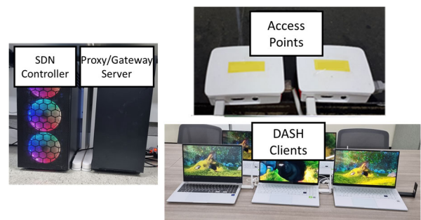
FIGURE 14. Real Wi-Fi testbed for the proposed HAS system.
