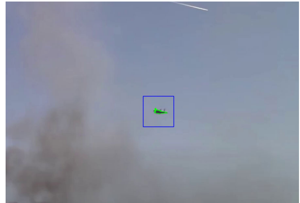
FIGURE 2. Considering Video 1 in experiments, this figure shows a target aircraft. The straight line segments detected using the probabilistic hough line transform are depicted with green line segments. A bounding box (blue box) is generated at the aircraft.
