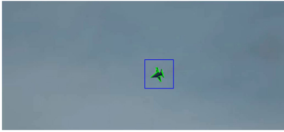
FIGURE 3. Considering Video 2 in experiments, a bounding box is generated at a target aircraft which is far from the camera. The straight line segments detected are depicted with green line segments.
