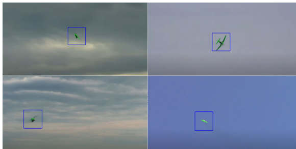
FIGURE 6. This plot shows the examples of a bounding box generated at various target aircrafts (Section III-A). The straight line segments detected using the probabilistic hough line transform are depicted with green line segments. See that our bounding box is generated on various kinds of aircrafts, including helicopters.
