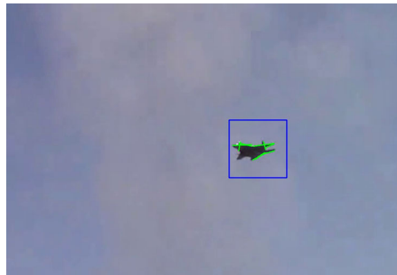
FIGURE 7. Considering Video 3 in experiments, this plot shows the bounding box formed at the target aircraft. The straight line segments detected using the probabilistic hough line transform are depicted with green line segments.
