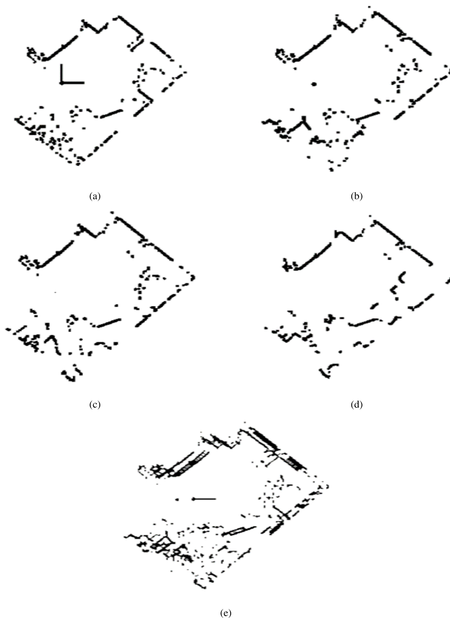
FIGURE 20. Processed images of maps given in Fig. 24 created using surrounding environment. Each image consist with spatial information about the obstacle in different levels of heights. lowest ground covers by (a) and highest ground is shown in (d) (b) and (c) depicts the middle layers. (e) shows the complete image after overlapping all the 4 layers. Overlapped image is used to enhance and identify boundaries and obstacles. Visual image of the environment is given in Fig. 24.
