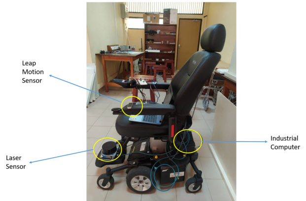
FIGURE 10. Wheelchair setup used for the human studies and the experiments.
