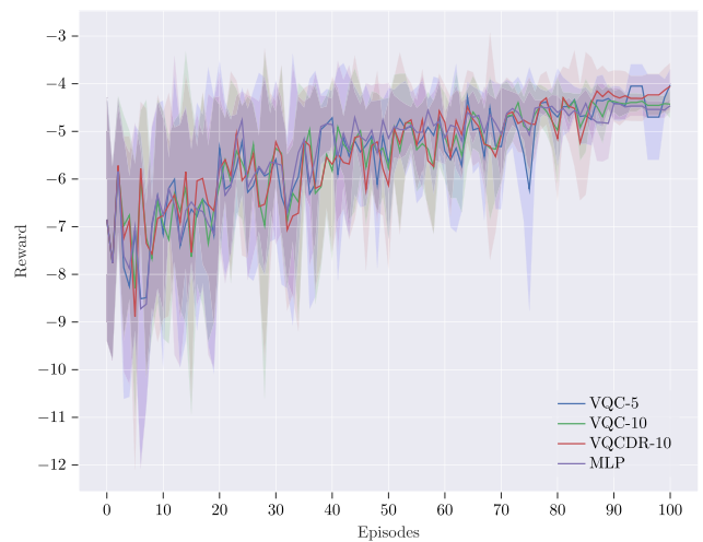
FIGURE 15. Learning curves obtained from four distinct methods in Use case 2. The approaches are: VQC with Amplitude Encoding using 5 qubits, VQC with a linear layer at pre-processing, a variant of the latter approach which incorporates data-reuploading and scaling methods, and the use of MLP.
