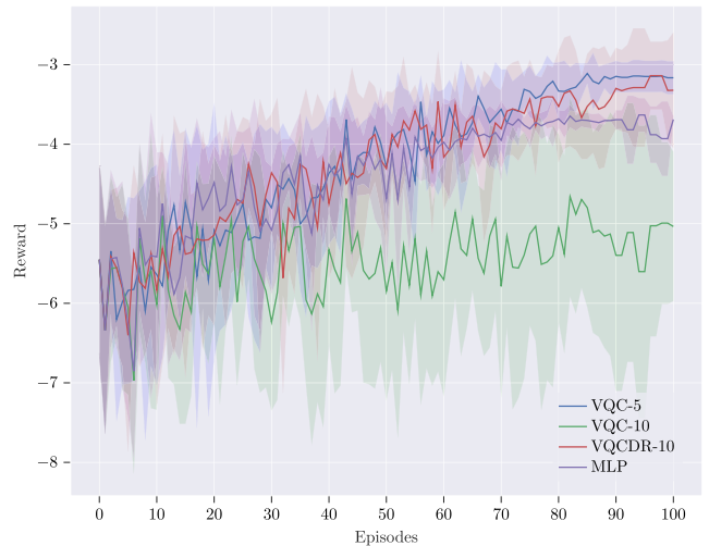
FIGURE 12. Learning curves obtained from four distinct methods in Use Case 1. The approaches are: VQC with Amplitude Encoding using 5 qubits, VQC with a linear layer at pre-processing, a variant of the latter approach which incorporates data-reuploading and scaling methods, and the use of MLP.
