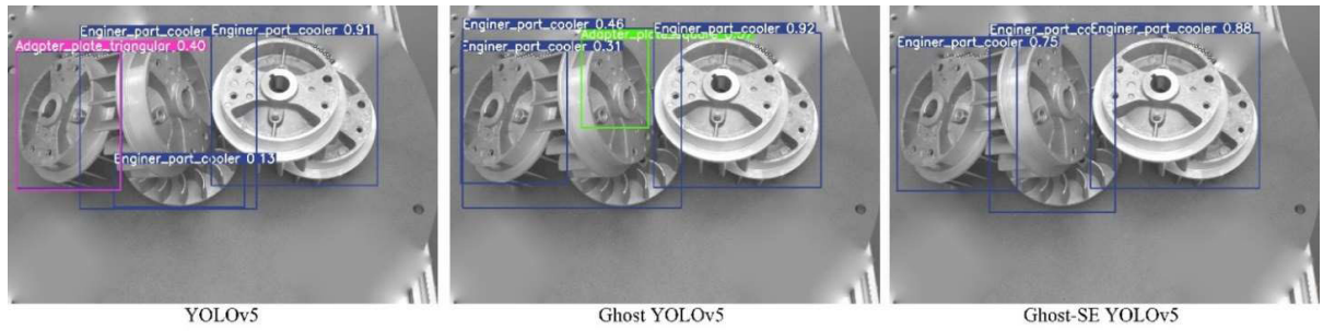
(a) The results of engine cooling parts identification and positioning
