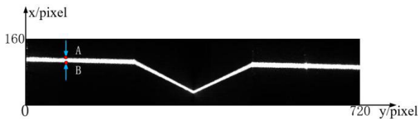
FIGURE 6. The principle of the row-by-row (column) search method.
