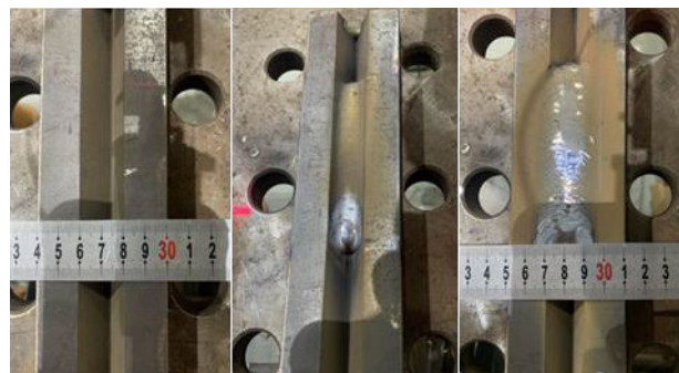
(a) Before welding (b) During welding (c) Finish welding
