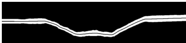
FIGURE 14. The skeleton line of the weld image.
