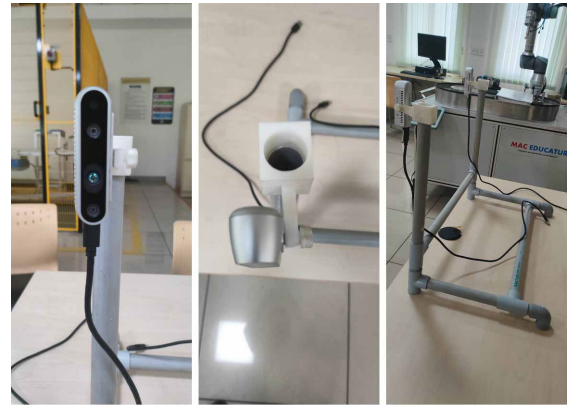
(a) Camera 1 (b) Camera Holder Top view (c) Camera setup side view
