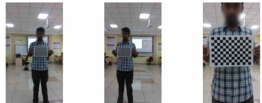
(a) Stereo Calibration Frame for Camera 0 (b) Stereo Calibration Frame for Camera 1 (c) Mono Calibration Frame for Camera 0
