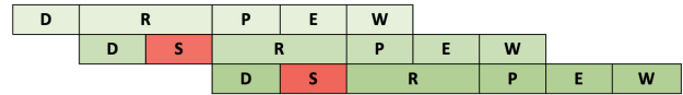
FIGURE 8. The different stages of the pipeline: [D]iscovery, [R]eading, [P]arsing, [E]laboration, [W]rite-Back. In a realistic scenario, some [S]talls might be present.
