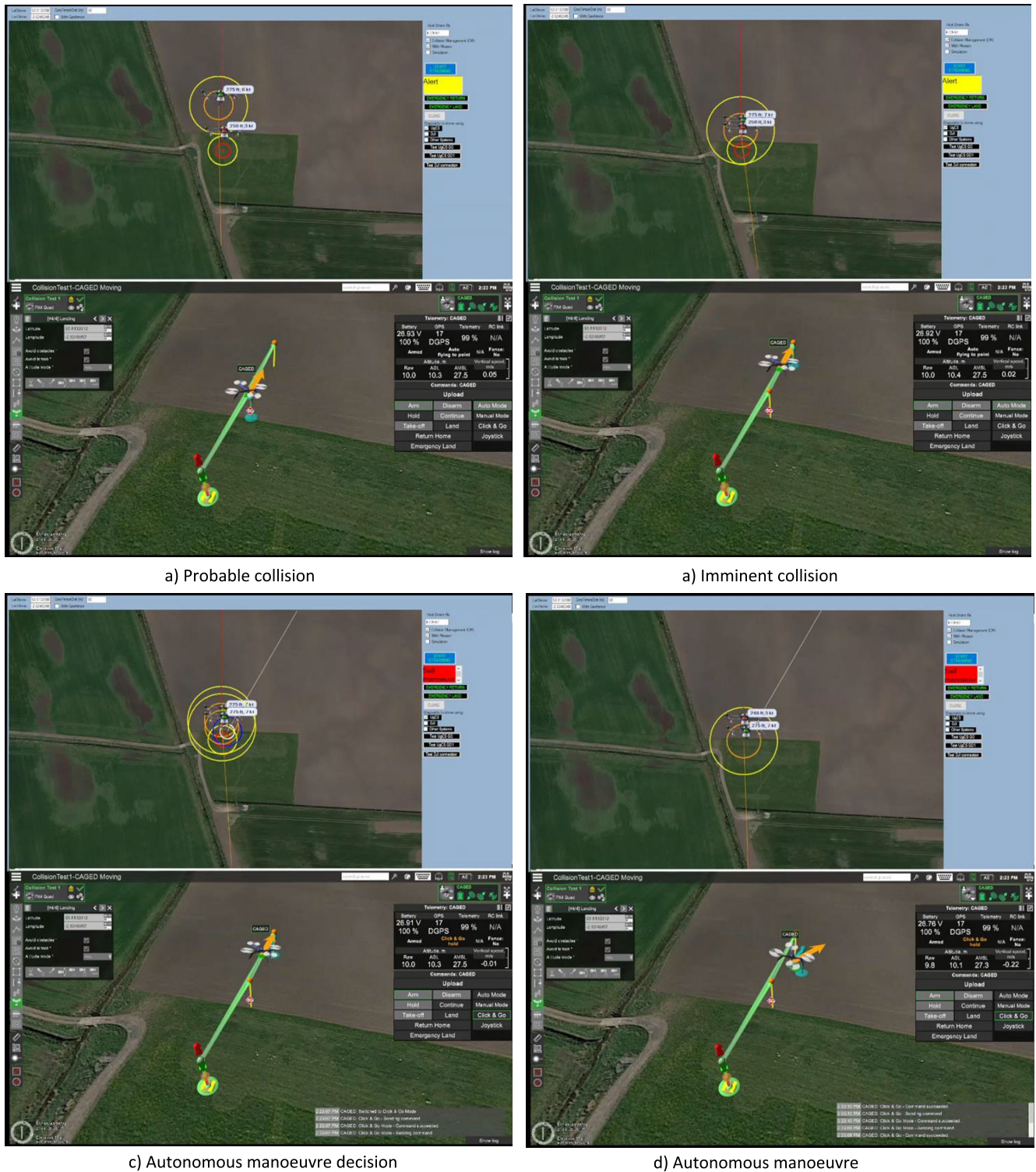
FIGURE 15. Real field tests: Top images show the screenshots of the developed application whereas the bottom images show the UgCS control system at a time where the UgCS system is responsible for executing the modified control commands. The red circles indicate the spherical ICTZones of meD and the brown circles indicate the ICTZones of the other flights in the environment; the yellow circles correspond to the spherical PCTZones of flights. The circles for the autonomous successive course of manoeuvres of meD turn into white ICTZone and heading and blue PCTZone as shown in c and d.
