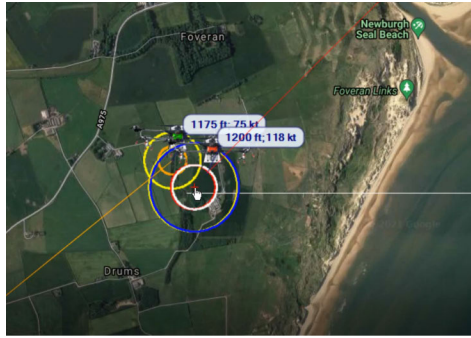
FIGURE 10. Geometric illustration of CA manoeuvres with Alg. 5. meD.MoveDistance is corresponding to the invasion length of ICTZones (Table 8).
