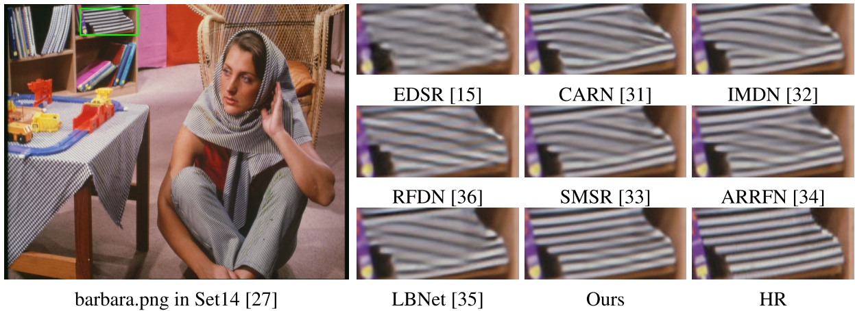
FIGURE 7. The green rectangle marks a 118 \times 52 \times 3 patch from barbara.png in the dataset Set14 [27]. On the right side are its \times 4 super-resolution results, and the names of the corresponding super-resolution algorithms are marked below the results. HR is the high resolution patch, or known as the ground truth.
