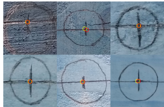
FIGURE 10. Regression outcomes from utilizing ShuffleNet on the testing subset, where red represents ground truth and yellow indicates predicted values.
