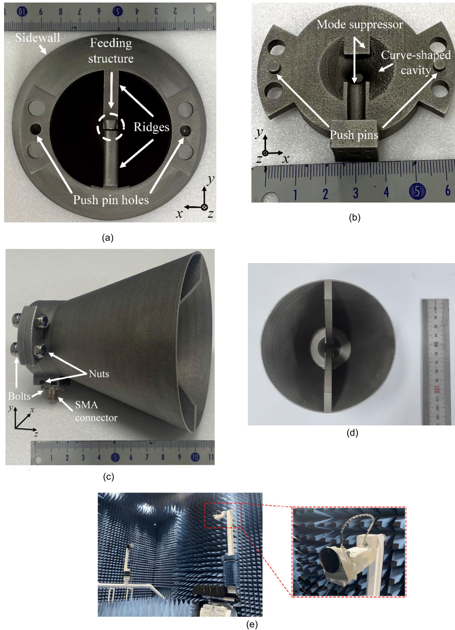
FIGURE 2. Photographs of the fabricated antenna. (a) Flare part. (b) Cavity part. (c) Proposed antenna (side view). (d) Proposed antenna (front view). (e) Measurement setup.
