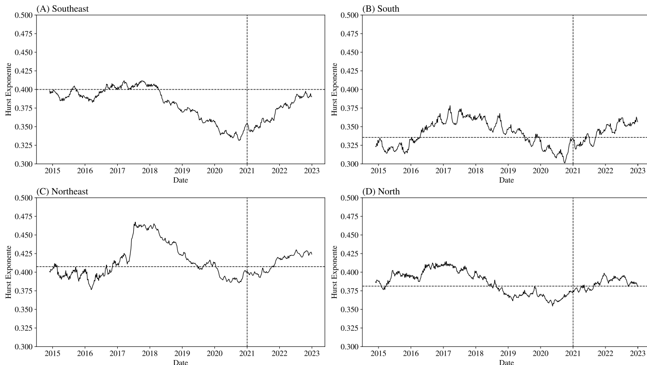
FIGURE 7. The graphs present the dynamic behavior of the Hurst coefficient ( H_2 ) for the four submarkets using a window of 702 weeks and a unit step. The dashed vertical line indicates when there was a transition in how the price was calculated, with the introduction of the hourly hydrothermal dispatch model on January 1, 2021. Before this date, the price was calculated weekly through a weekly hydrothermal dispatch model. From this landmark, the weekly price started to be obtained by the arithmetic average of the hourly prices throughout the week. The dashed horizontal line represents the value of H_2 calculated for the complete series, as presented in Table 3.
