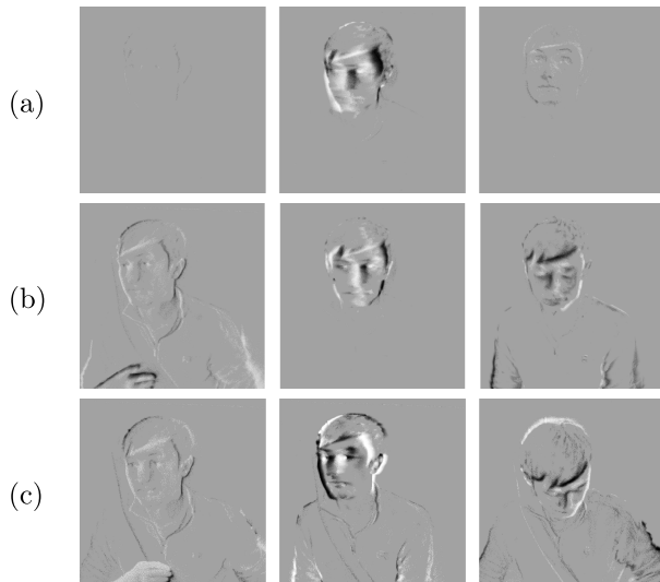
FIGURE 6. A “Seatbelt fastened” clip that was converted from events to frames using (a) a fixed time period, (b) a fixed event count, and (c) a fixed event count over the torso region with a minimum duration, so that each method yields 75 frames total. Of these 75 frames, the seatbelt was visible in (a) 27%, (b) 71%, and (c) 93%.
