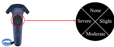
FIGURE 3. Illustration of the coordinate-segmentation method using the HTC Vive controller trackpad for 4-level CS evaluation.
