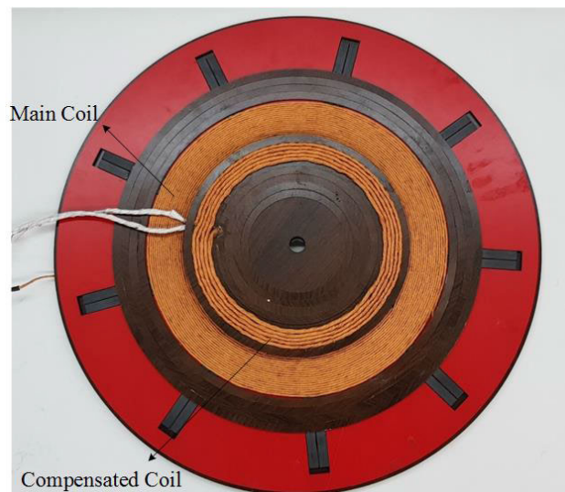
FIGURE 10. The experimental coil structure.
