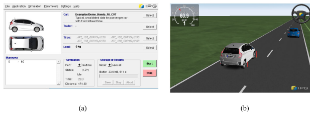
FIGURE 2. The IPG CarMaker® environment for vehicle and traffic simulation. (a) Initial screen with options for configuring simulation parameters. (b) IPGMovie® interface for visualising vehicle manoeuvres in real-time.
