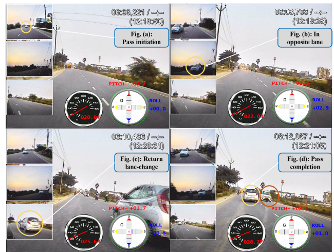
FIGURE 8. (a) Initiation of overtaking manoeuvre, (b) Completion of outgoing lane change, (c) Start of incoming lane change after passing the probe vehicle, (d) Completion of overtaking manoeuvre in the face of oncomer.
