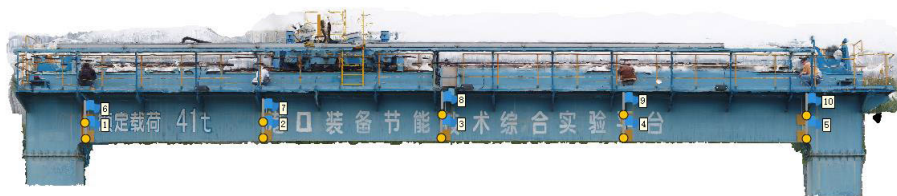
FIGURE 31. Point cloud model of the main girder after deformation.
