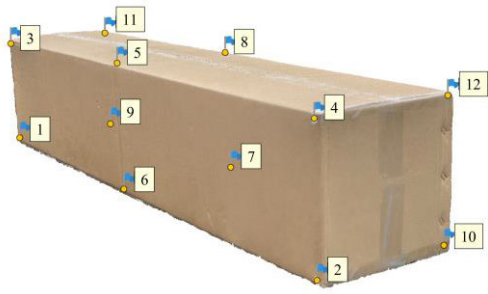
FIGURE 14. The reference point cloud model constructed under full control and marker point layout.
