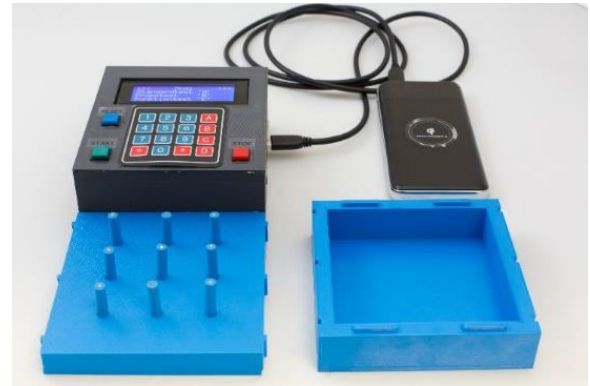
FIGURE 1. The components of the dNHPT (test board with control unit, peg container and voltage supply).
