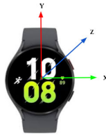
FIGURE 15. The three axes of a smartwatch.
