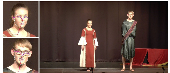
FIGURE 23. Detection of lip movements with OpenPose based on the difference of the y-values of the upper lip and lower lip.
