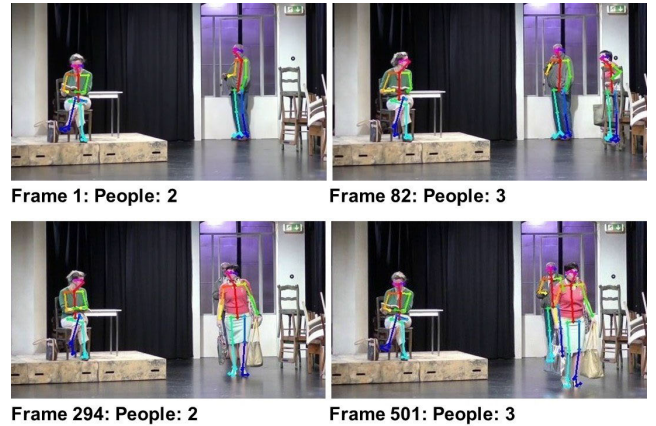
FIGURE 10. Occlusion: If one person is in front of another, only one person is detected.
