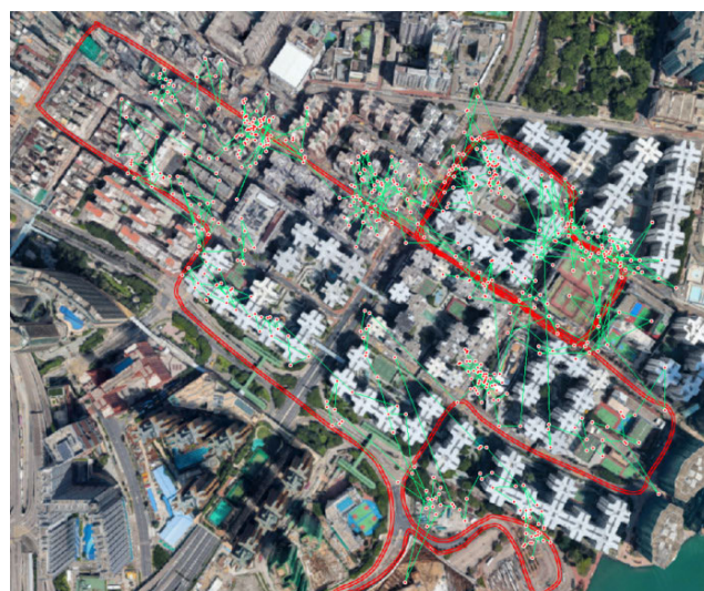
FIGURE 8. GNSS position track after RTK processing. The red line indicates the reference trajectory.
