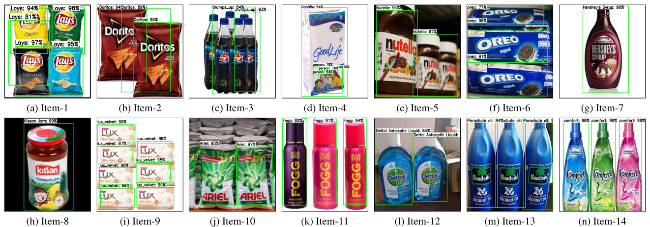
FIGURE 2. SSD based object detection for selected items (14 out of 40) during training phase.
