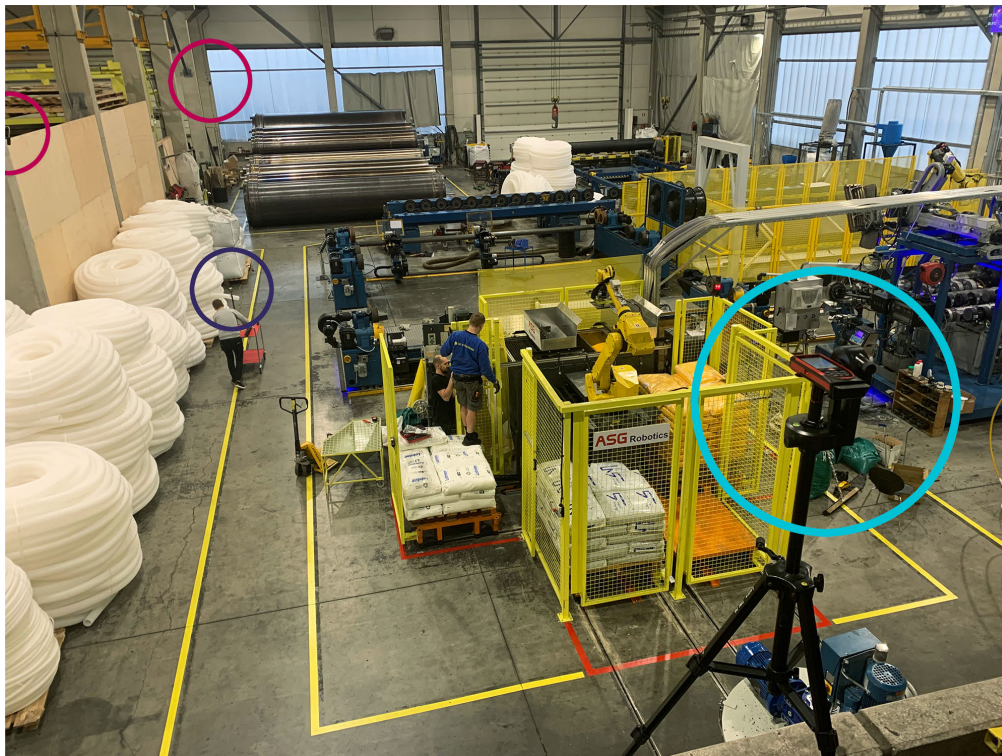
FIGURE 3. Setup for the movement tests in the industrial environment. Visible anchors A_1 and A_6 are circled in red, the Leica DISTO S910 in cyan, and the tripod-mounted tag on the shelf trolley in dark blue. The tag is moved in reference to the lines on the factory floor.
