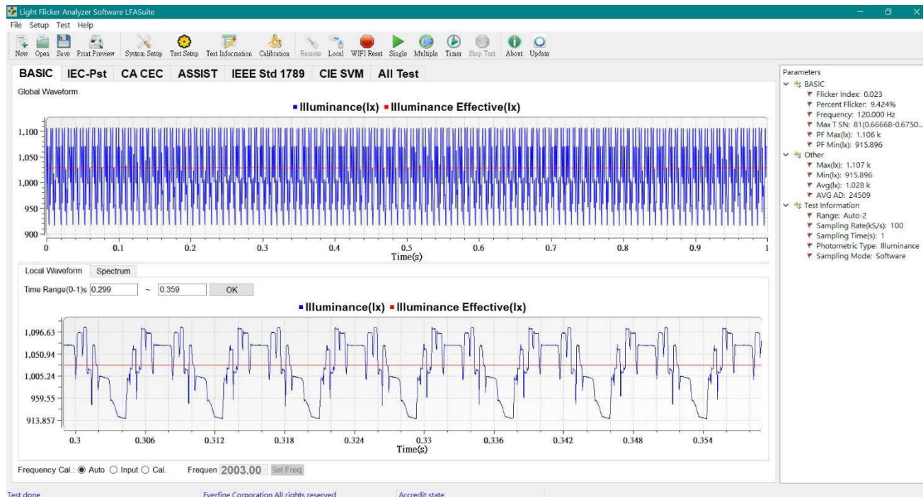
FIGURE 11. Measured percentage flicker of the proposed linear converter.
