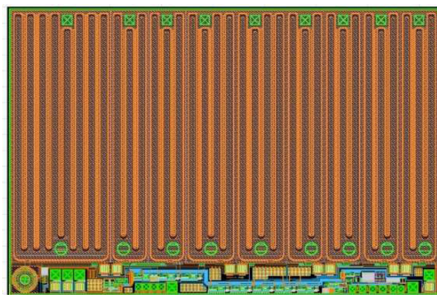
FIGURE 9. Layout of the adopted IC.
