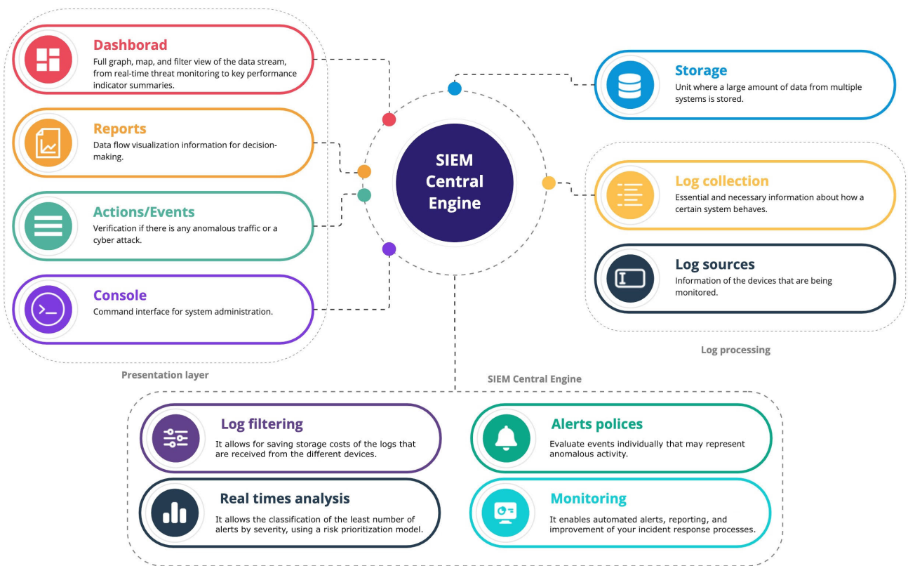
FIGURE 2. Physical architecture of the SIEM.
