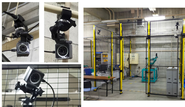
FIGURE 8. Motion capture system attached to crane environment.
