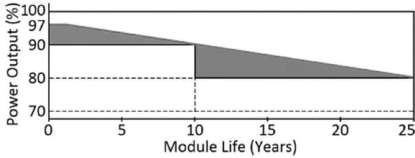
FIGURE 5. The lifespan graph of typical solar PV modules [14].
