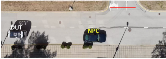
FIGURE 18. Passing scenario setup. The entrance to the T intersection was blocked to avoid interruption.
