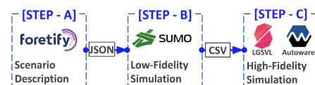
FIGURE 2. Three main steps of the proposed validation method. The format of each signal passing among these steps is annotated.
