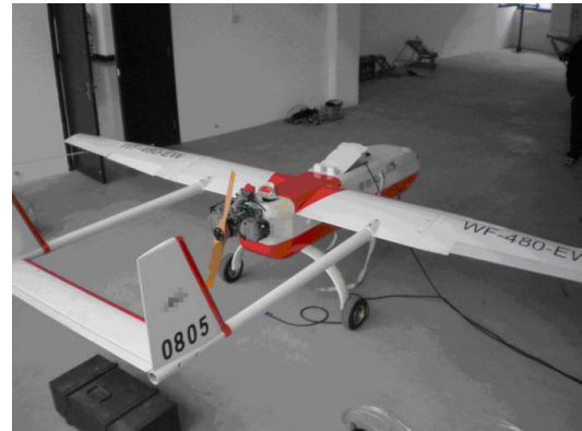
FIGURE 9. Aircraft used for flutter experiment.
