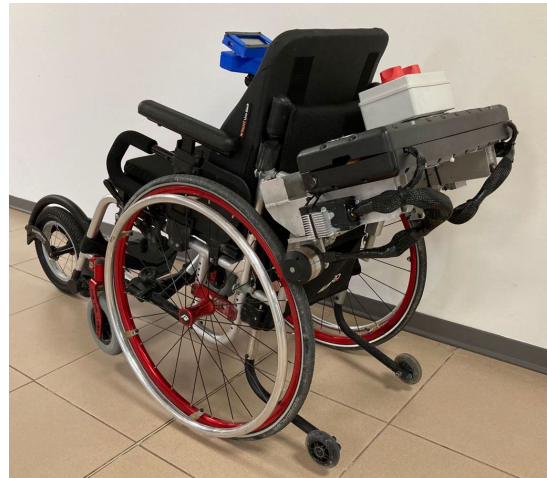
FIGURE 22. Wheelchair with plug-and-play kit.
