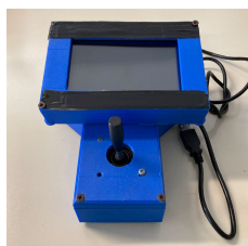
FIGURE 20. Subsystem joystick-screen-MCU with USB cable for power supply.
