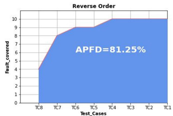
FIGURE 7. APFD value of fault detected by 'reverse ordering'.
