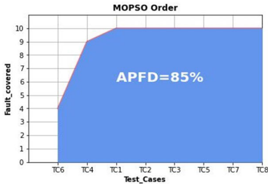
FIGURE 8. APFD value of fault detected by the proposed approach.
