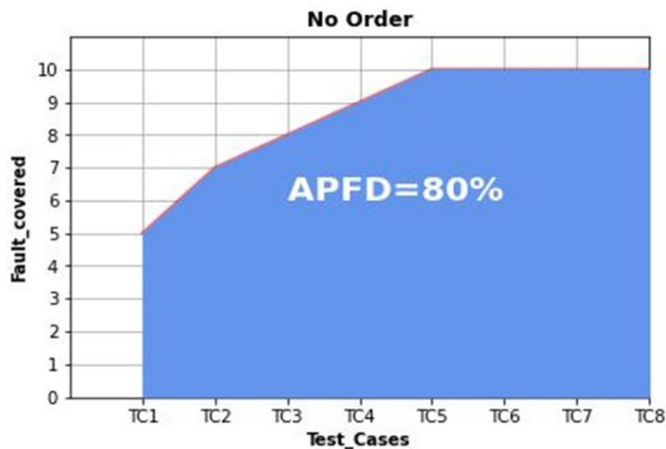
FIGURE 5. APFD value of fault detected by 'no ordering'.
