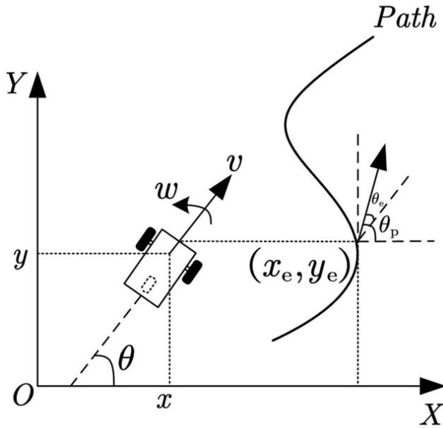
**FIGURE 2.** Path planning schematic of the mobile manipulator. (All variables are marked with black symbols, where the thick black arc represents the path.)
