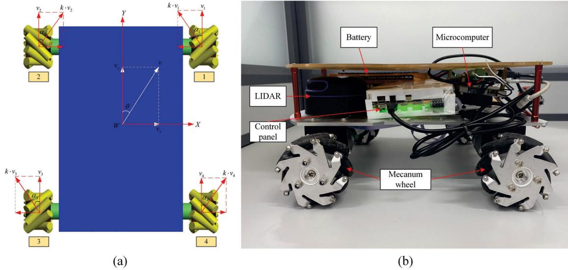
**FIGURE 1.** The mobile robot experimental equipment of the actual physical manipulator is displayed via a mobile base model. (a) Mobile base coordinate system (for kinematic analysis); (b) Mobile base (for providing power).
