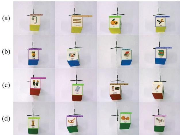
**FIGURE 7.** Results display for object detection. (a) Yellow block objects; (b) Blue block objects; (c) Red block objects; (d) Green block objects. (Object detection is marked with different color boxes and text, respectively.)
