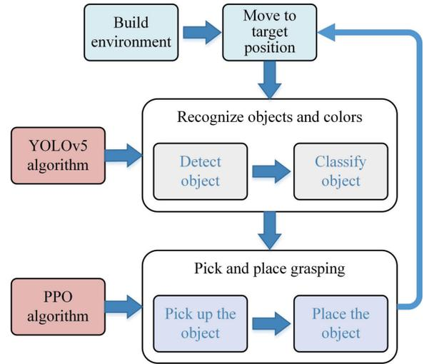
**FIGURE 3.** The interaction structure of the vision algorithm and grasp algorithm where the mobile manipulator interacts with the objects.
