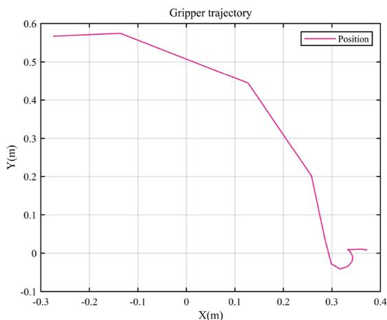
**FIGURE 11.** The position trajectory of the manipulator's gripper corresponds to the trajectory in Fig. 10 (f). (Position trajectory is marked with a pink line.)
