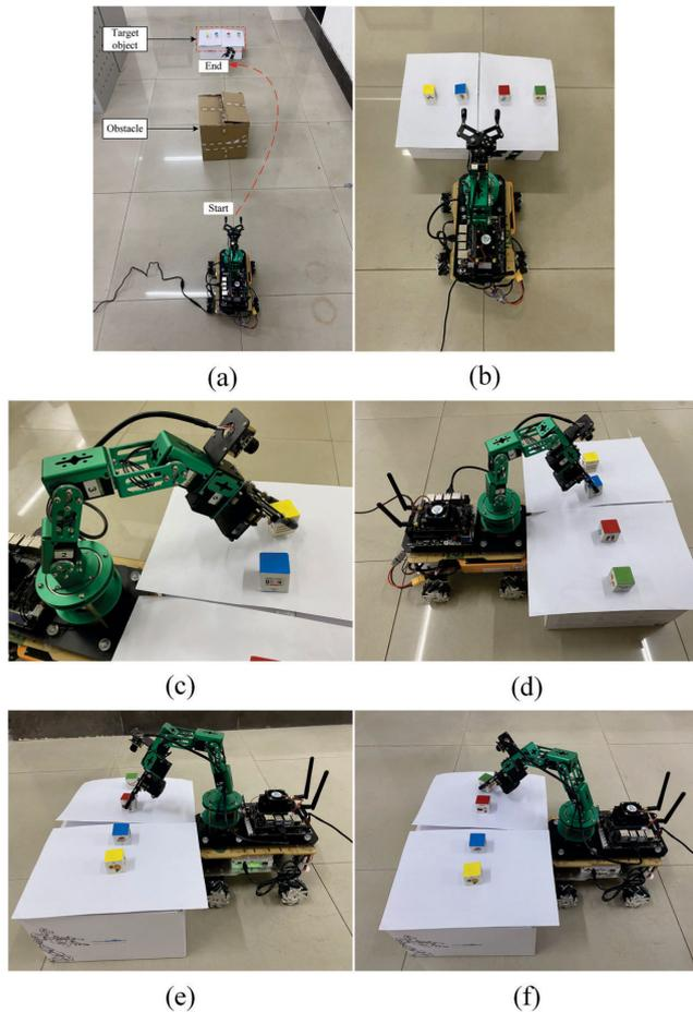
**FIGURE 14.** The grasping experiment scene in the real world. (a) Move the manipulator to the target point; (b) Mobile manipulator reaches the gripping platform; (c) Grasping the yellow block; (d) Grasping the blue block; (e) Grasping the red block; (f) Grasping the green block. (Four experimental color blocks are placed on the gripping platform.)
