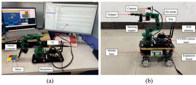
**FIGURE 13.** The experimental platform for object recognition and grasping. (a) Experimental platform setup; (b) The Physical model of the DOFBOT mobile manipulator. (The hardware devices of the mobile manipulator are marked with red arrows, respectively.)
