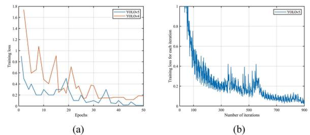
**FIGURE 9.** The training loss of the YOLOv5 algorithm. (a) Loss comparison between the YOLOv5 and YOLOv4 algorithms; (b) Training loss for each iteration of the YOLOv5 algorithm. (YOLOv5 and YOLOv4 algorithms are marked with the blue line and Orange line, respectively.)
