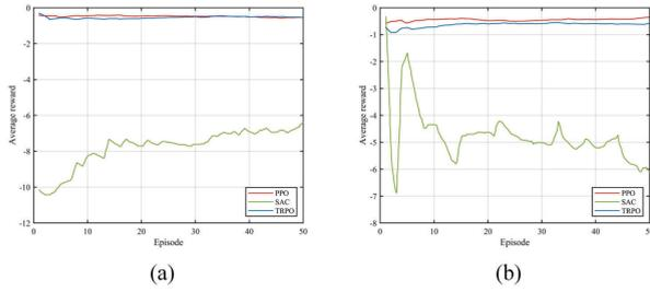
**FIGURE 12.** The average reward comparison of the PPO, SAC, and TRPO algorithms. (a) Average reward curve at batch 16; (b) Average reward curve at batch 128. (PPO, SAC, and TRPO algorithms are marked with red, green, and blue lines, respectively.)
