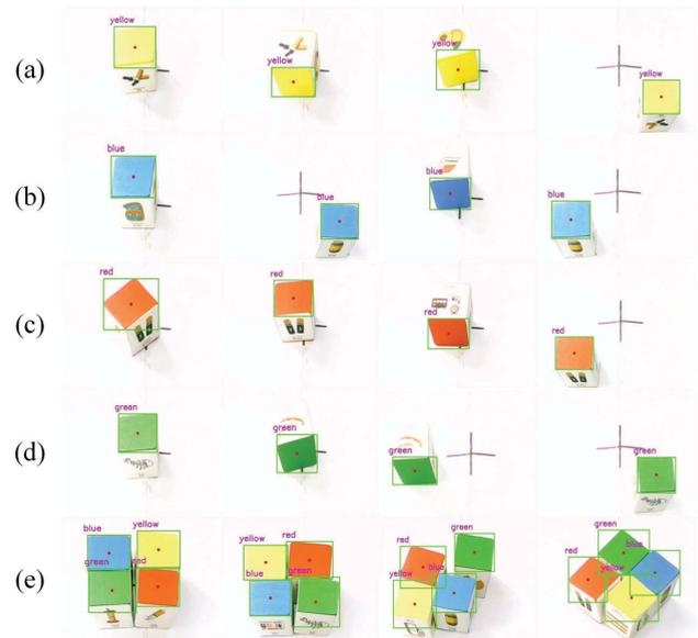
**FIGURE 6. Results display for color detection. (a) Yellow color; (b) Blue color; (c) Red color; (d) Green color; (e) Four blocks colors. (Color detection is marked with a green box and purple text, respectively.)**
