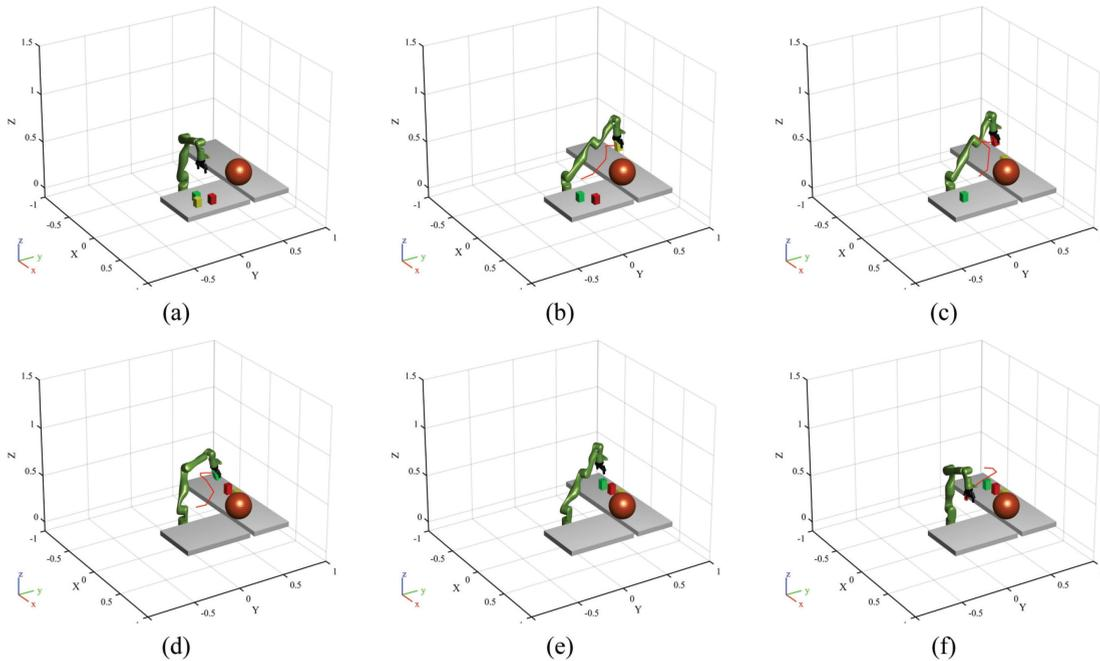
**FIGURE 10.** The trajectory results of object grasping via the PPO algorithm. (a) Start grasping; (b) Grasping the yellow block; (c) Grasping the red block; (d) Grasping the green block; (e) Finish grasping; (f) Reset manipulator's gripper. (Trajectories are marked with red line.)
