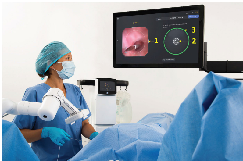
FIGURE 1. The guided percutaneous access interface (GPAI) of the Monarch Platform Urology (Auris Health Inc., CA). The interface consists of the ureteroscope camera view (1), target and targeting dot (2) that encodes the alignment between the needle for percutaneous insertion and the target inside the kidney, and depth indicator (3) that turns green when the target is reached or red when the target is missed.
