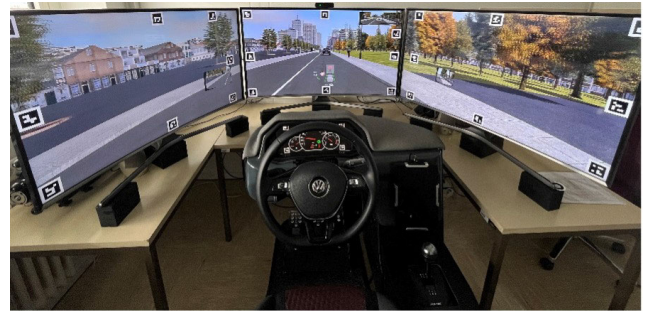
FIGURE 1. Nervtech motion-based driving simulator with a physical dashboard and 145° field of view of the driving environment.
