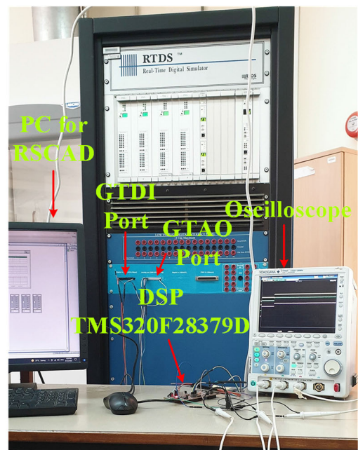
FIGURE 15. RTDS setup used to capture CHIL results of dc microgrid at Qatar University.
