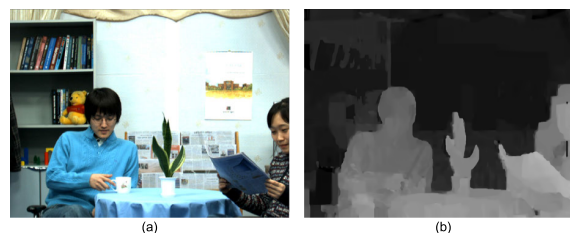
FIGURE 2. A frame from the video sequence "Newspaper" (a) texture map (b) depth map.
