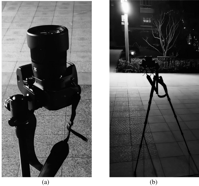
FIGURE 18. Star sensor and environment of the night sky experiments. The camera is mounted on a tripod with the lens facing up. In order to verify the robustness of the proposed algorithm, the environment with heavy light pollution and more noise is selected.
