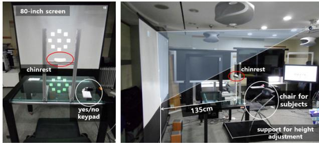
**FIGURE 1.** Depiction of the experimental environment. The distance between participants and projected screen is 135 cm. They stare at the center of the screen during the experiment. The resolution of the projected screen is 1024 × 768.
