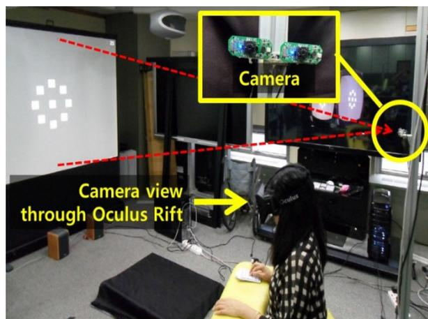
**FIGURE 3.** In VSHMD condition, participants saw the screen only through cameras mounted at 135 cm away from the projected screen, which is the same as the BLD and Bare eye condition.
