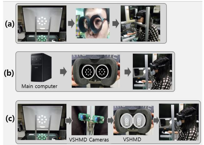
**FIGURE 2.** Viewing conditions and the devices used. (a) bare eye with blinder glasses (BLD), (b) stimuli displayed directly on head-mounted display (HMD), and (c) video see-through display in HMD (VSHMD).
