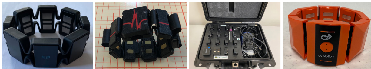
FIGURE 4. The supported hardware (at time of submission). From left to right, the (1) Myo Armband, (2) SIFI Labs Bioarmband, (3) Delsys Trigno and Avanti, and (4) gForcePro+ EMG Armband.
