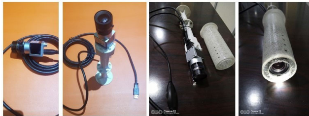
FIGURE 9. Camera and lens mounted on the probe body with LED light source attached.
