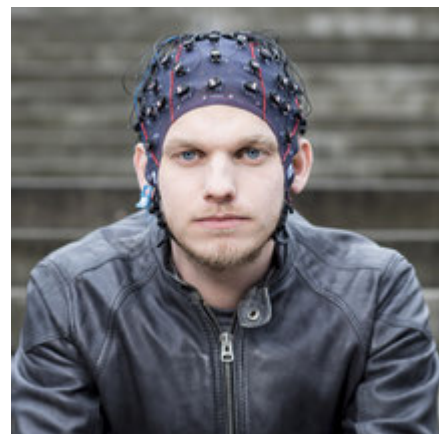
FIGURE 4. An advanced wearable EEG head cap [109]. The headcaps normally have a minimum of 8 electrodes with some advanced caps containing 256 electrodes. 32 electrodes have been found to be optimal for research purposes.
