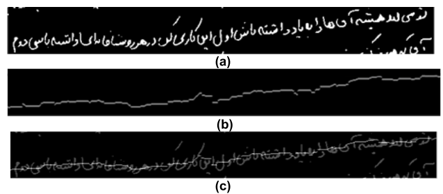
FIGURE 5. Extraction of baseline curve from a handwriting, a) a bonding box of a handwritten line, b) the extracted baseline curve, c) handwriting sample and its extracted baseline.
