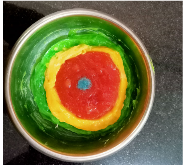
FIGURE 4. Fabricated heterogeneous breast phantom with tumor in a mould with skin (green), fat (yellow), gland (red), and tumor (blue) layers.
