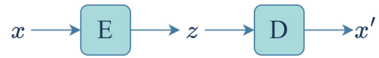
FIGURE 2. Input raw data x to train encoder E, whose output z is used to train decoder D and generate data x'.
