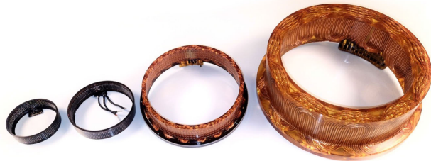
FIGURE 5. Examples of FiberPrinted stators in different sizes.
