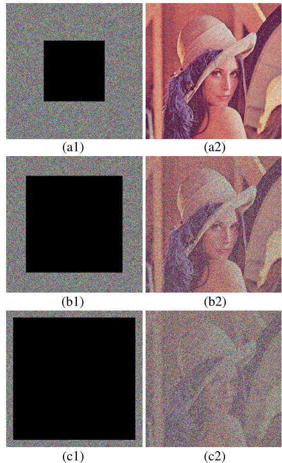
FIGURE 22. Resilience to occlusion attacks of optimal chaotic map under uni-s scheme, (a1) ciphertext blocked by 20 %, (b1) ciphertext blocked by 50 %, (c1) ciphertext blocked by 80 %, (a2) decrypted image from (a1), (b2) decrypted image from (b1), (c2) decrypted image from (c1).
